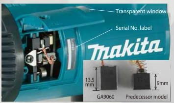
Change from basic spring to Spiral spring without losing the compact body yet extending the service life of Carbon brush.
