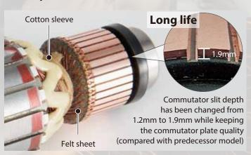
The fixing strength of coil has been significantly improved by adding cotton sleeve and felt sheet.
